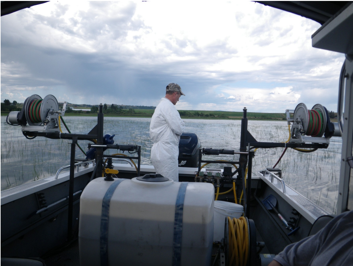
Figure 1. Water column injection of herbicides for suppression of flowering rush in East Bay Flathead Lake.
